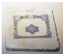
A lithographic printing plate (a stock certificate)
